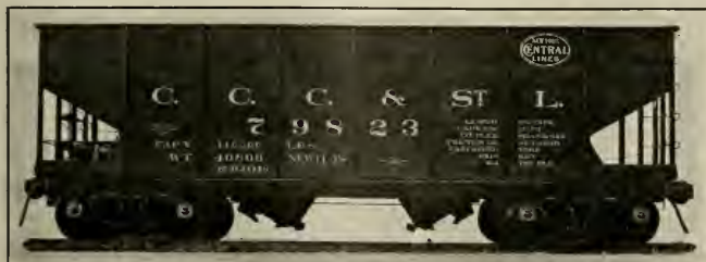
55-TON TYPE OF STEEL HOPPER CAR FOR THE CLEVELAND, CINCINNATI, CHICAGO & ST. LOUIS RAILROAD.
